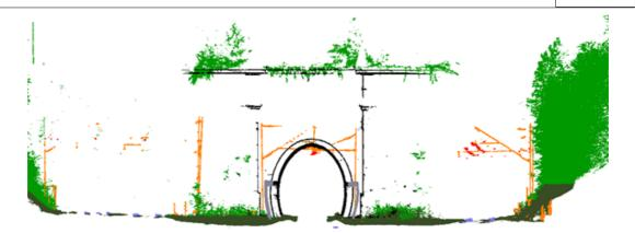
By selecting and isolating appropriate elevation and sectional areas, the user can quickly differentiate the tunnel, cabling, rails, and foliage. This in turn allows the user to cut complex sections, develop a ground surface and isolate features of interest.
